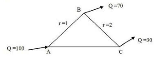
The head loss in each pipe is given by  $h_f = rQ^{1.8}$ , with the variables expressed in a consistent set of units. The value of r for the pipe AB is 1 and for the pipe BC is 2. If the discharge supplied at the point A (i.e., 100) is equally divided between the pipes AB and AC, the value of r (up to two decimal places) for the pipe AC should be
