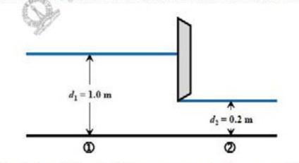
A sluice gate used to control the flow in a horizontal channel of unit width is shown in the figure.
