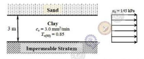
For the given ground conditions, the time (in days, rounded to the nearest integer) required for 90% consolidation would be
