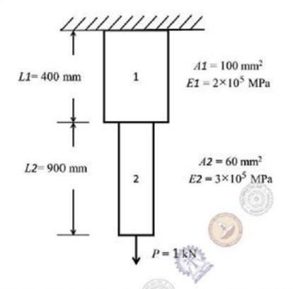
Segments 1 and 2 have cross-sectional area of  $100 \text{ mm}^2$  and  $60 \text{ mm}^2$ , Young's modulus of  $2 \times 10^5 \text{ MPa}$  and  $3 \times 10^5 \text{ MPa}$ , and length of 400 mm and 900 mm, respectively. The strain energy (in N-mm, up to one decimal place) in the bar due to the axial load is \_\_\_\_\_\_
