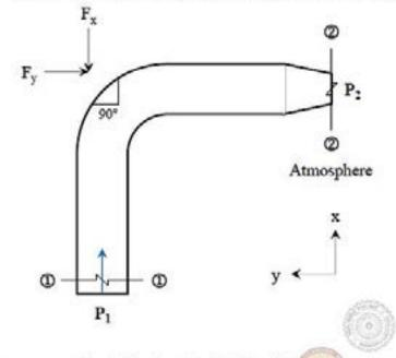
A pressure of 140 kPa is measured at Section 1-1. The inlet diameter marked at Section 1-1 is  $\frac{27}{\sqrt{\pi}}$  cm, while the nozzle diameter marked at Section 2-2 is  $\frac{14}{\sqrt{\pi}}$  cm. Assume the following:
